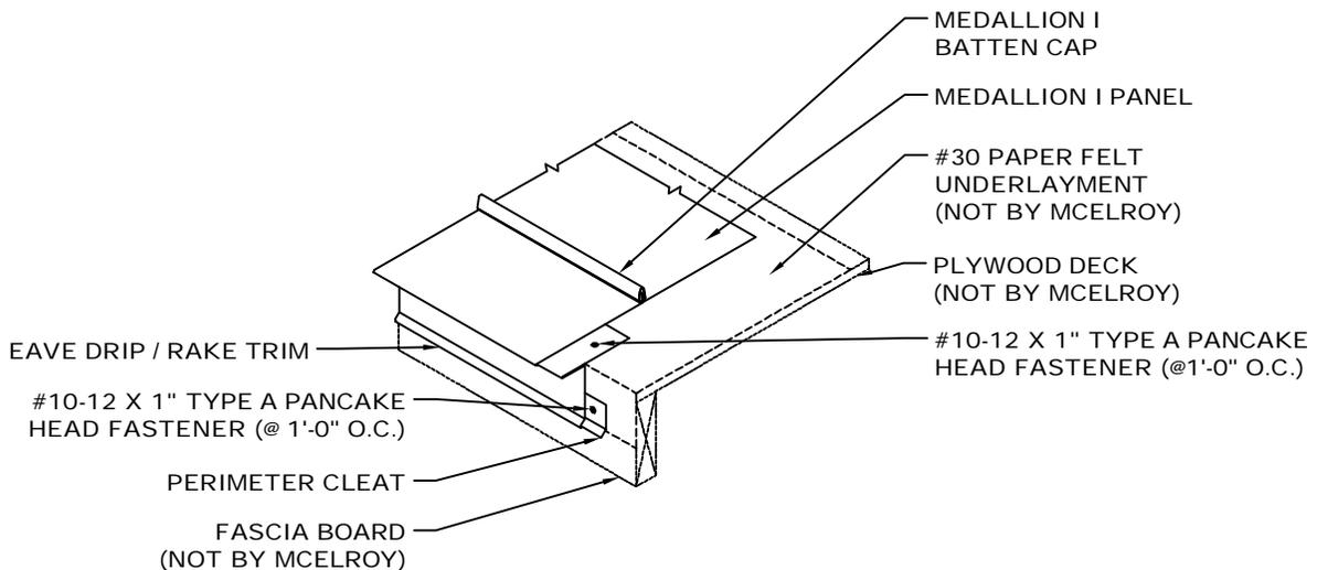
\*NOTE: SOME TRIM ITEMS AND FASTENERS HAVE BEEN REMOVED FOR CLARITY OF ISOMETRIC DETAIL.
