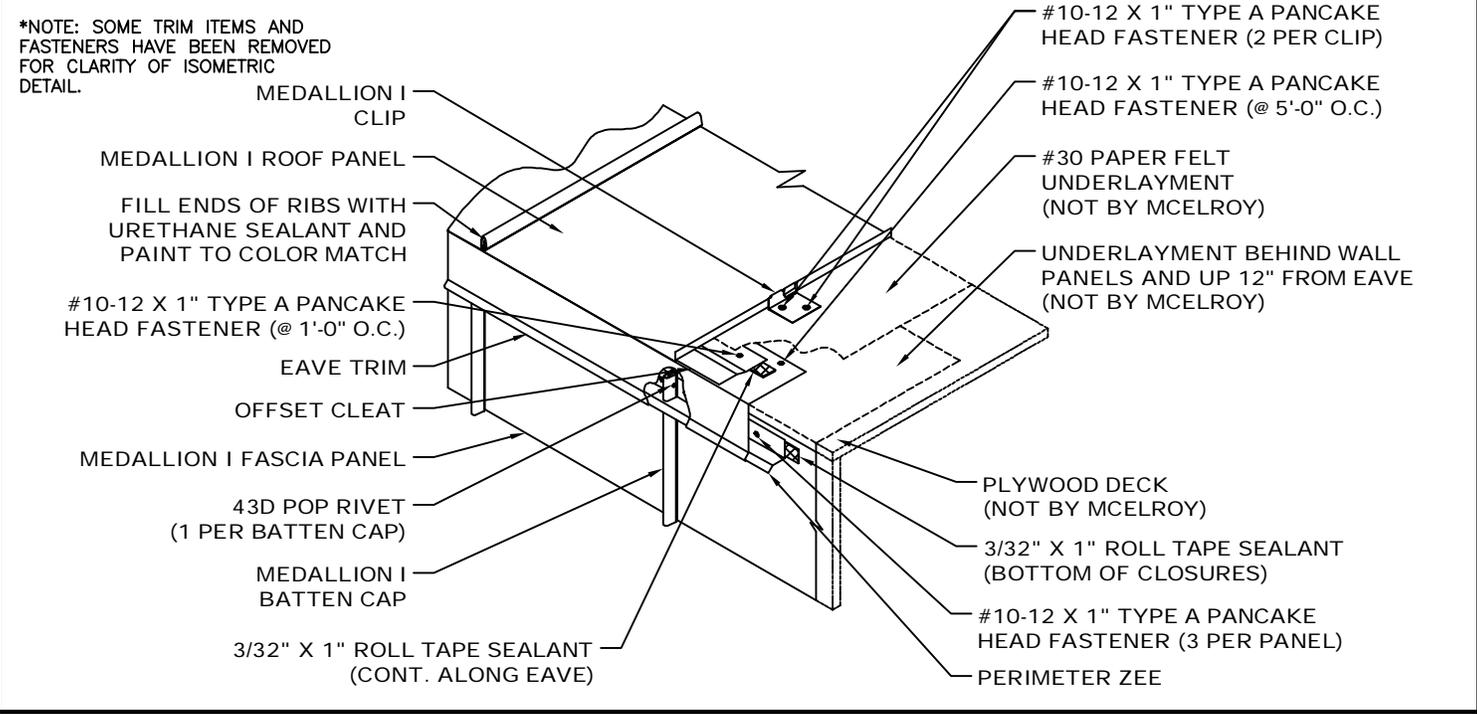
\*\* CLEARANCE REQUIRED FOR THERMAL MOVEMENT
