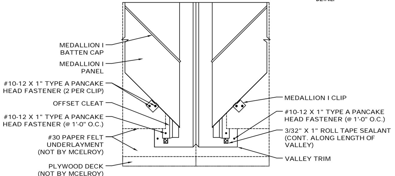
**\*\* CLEARANCE REQUIRED FOR THERMAL MOVEMENT**
